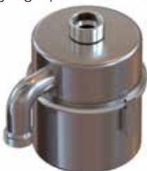
Sediment traps stop the residues that are otherwise flushed out via the outlet and risk causing blockages in the drain pipes. Usually placed in connection with stainless steel workbenches and wash troughs. Solid particles are separated from the water and remain at the bottom of the container.
