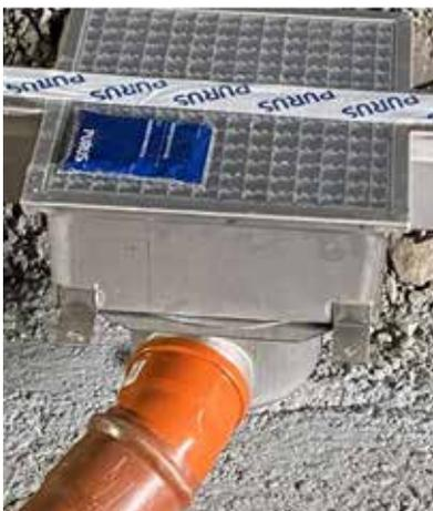
Our floor channels and gullies are made of acid-resistant stainless steel (EN 1.4404), which provides high chemical resistance. Even loose parts such as water traps are made of acid-resistant steel. The picture shows a 110 mm side outlet, also available as bottom outlet. The capacity over the water trap and filter bucket is 5.5 l/s, diverting large quantities of water.
