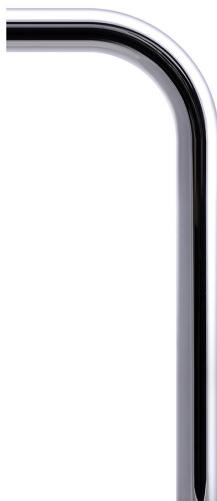
32mm chromed 90° pipe with smooth end on both sides for surface piping. Length 160x600mm, can be cut to the desired length. Made of ABS, which can be glued.
