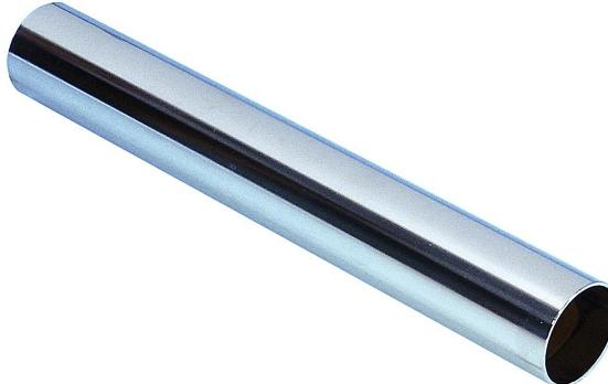
32mm chromed straight pipe with smooth end on both sides for surface piping. Length 950mm, can be cut to the desired length. Made of ABS, which can be glued.
