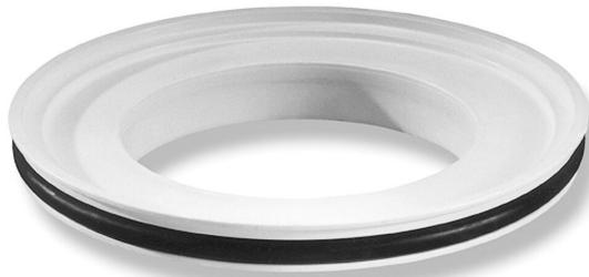
Adapter ring 220 is suitable for Purus floor drains with a grate diameter of 220mm. It is used to adapt 220mm diameter drains to a smaller diameter of 150mm, so that other water traps and grates can be used.
