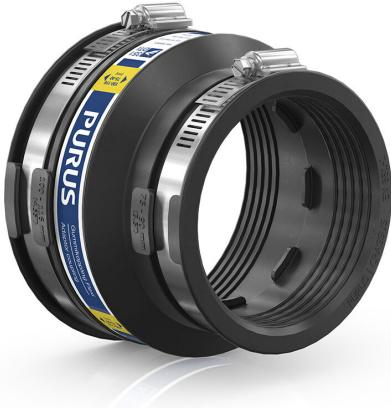
Adaptor couplings are used to connect two waste water pipes with different dimensions, as well as waste water pipes with the same or different materials and surface structure. Adaptor couplings are suitable for vertical and horizontal installation. They have two sides, both with hose clamps for external installation of waste water pipes. They are easy to install in a few minutes and are approved for concealed placement. The material is UV-resistant.
