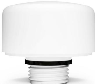
Air admittance valve  $\frac{1}{2}$ " is used for secondary air admittance, for example in drainage pipes. The air admittance valve 50/40 is installed with the intention of increasing the capacity and/or reducing the dimension.
