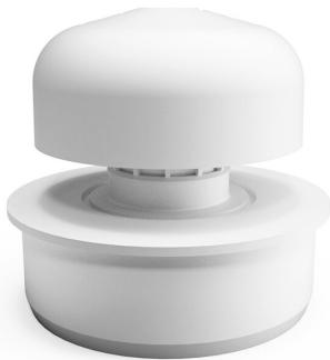
Air admittance valve 40 with adapters is used for secondary air admittance, for example in drainage pipes. The air admittance valve 40 is installed with the intention of increasing the capacity and/or reducing the dimension. The air admittance valve has an air flow capacity of 11.3l/s at a negative pressure of 250Pa. The air admittance valve is CE marked and meets the requirements of SS-EN12380 A1. Includes Styrofoam cover and adapter.
