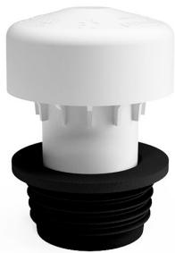
Air admittance valve 50/40 is used for secondary air admittance, for example in drainage pipes. The air admittance valve 50/40 is installed with the intention of increasing the capacity and/or reducing the dimension. The air admittance valve has an air flow capacity of 11.3l/s at a negative pressure of 250Pa. The air admittance valve is CE marked and meets the requirements of SS-EN12380 A1.
