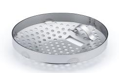
Filter bucket in acid-resistant stainless steel with a volume of 0.2 litres, designed to fit the Channel 200 and Square Top Gullies. The filter bucket is used to collect particles larger than 5mm, such as leaves, so they do not block the water trap. The filter bucket can be removed for emptying and cleaning.
