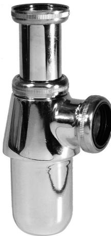
Bottle trap in chromed plastic for wash basin, 1¼" connection, designed to fit 40mm diameter outlet pipes. The bottle trap has a telescopic tube for adjusting the distance to the wash basin, as well as a removable base section for easy cleaning.
