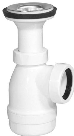
Bottle trap for wash basin, 1¼" connection, designed to fit 40mm diameter outlet pipes. The bottle trap has a flange, strainer and a removable base section for easy cleaning.
