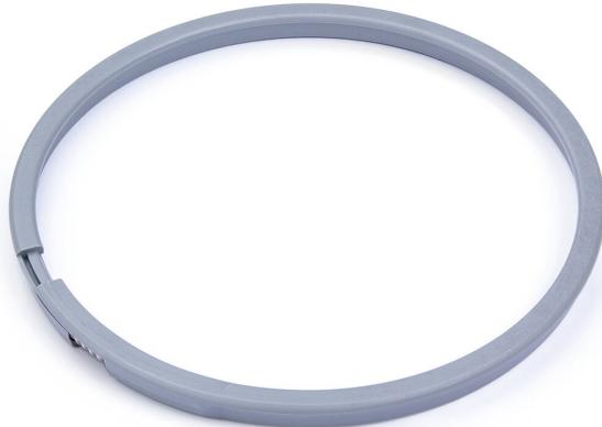
The Clamping ring automatic 220 is made of plastic, fitted with a spring and is used for both sealing membrane and vinyl flooring. It is a self-adjusting clamping ring for vinyl flooring with a thickness of 1,5 mm to 2 mm. Fits in Purus floor drains with grate dimension 220mm.
