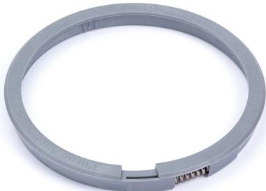
The Clamping ring automatic 130 is made of plastic, fitted with a spring and is used for both sealing membrane and vinyl flooring. It is a self-adjusting clamping ring for vinyl flooring with a thickness of 1,5 mm to 2 mm. Fits in Purus floor drains with grate dimension 150 mm.
