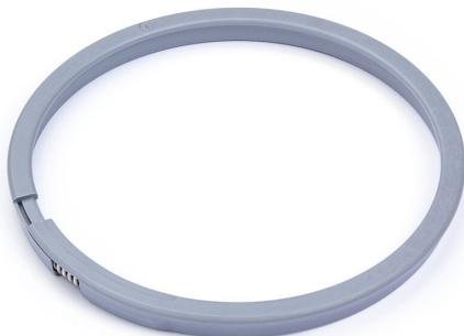
The Clamping ring automatic 150 is made of plastic, fitted with a spring and is used for both sealing membrane and vinyl flooring. It is a self-adjusting clamping ring for vinyl flooring with a thickness of 1,5 mm to 2 mm. Fits in Purus floor drains with grate dimension 150 mm.
