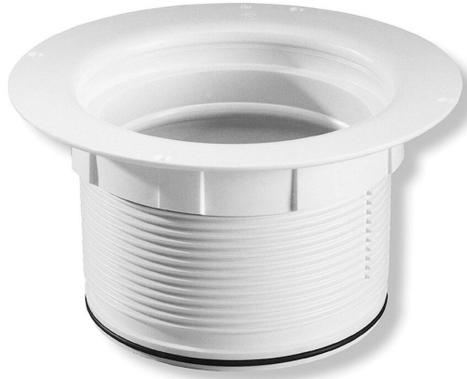
Flex extension ring in plastic with round flange, designed for Purus floor drains in plastic and cast iron with a grate dimension of 150mm. Comes with o-ring. The extension ring is used when you need to raise the flange, for example when levelling concrete. Raises 35-107mm and can be cut to size.
