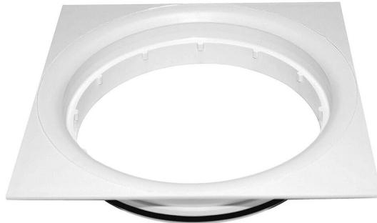
Extension ring 13 in plastic with square flange, intended for Purus floor drains in plastic and cast iron with a grate diameter of 150mm. Comes with o-ring. The extension ring is used when you need to raise the flange, for example when levelling concrete. Raises 13mm.
