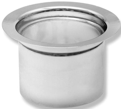
Extension ring 50 in acid-resistant stainless steel with round flange, intended for Purus' stainless steel floor drains with a grate diameter of 150mm. Comes with gasket. The extension ring is used when you need to raise the flange, for example when levelling concrete. Raises 50mm and can be cut.
