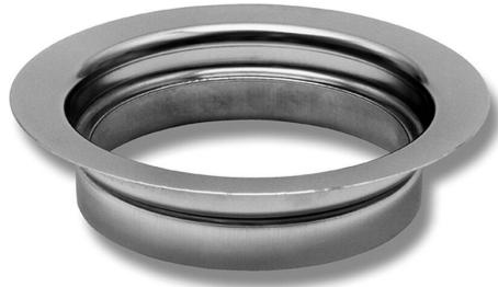
Extension ring 25 in acid-resistant stainless steel with round flange, designed for Purus' stainless steel floor drains with a grate dimension of 150mm. Comes with sealing gasket. The extension ring is used when you need to raise the flange, for example when levelling concrete. Raises 25mm.
