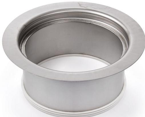
Extension ring 50 in acid-resistant stainless steel with round flange, intended for Purus' stainless steel floor drains with a grate diameter of 220mm. Comes with gasket. The extension ring is used when you need to raise the flange, for example when levelling concrete. Raises 50mm and can be cut.
