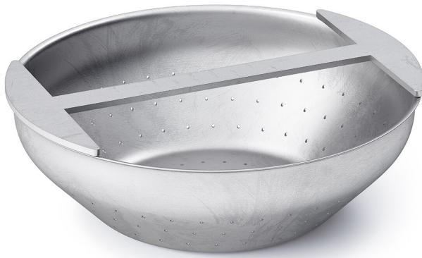
Filter bucket BH50 in acid-resistant stainless steel with a volume of 1.1 liters. The filter bucket is used to collect particles larger than 2 mm, e.g. fish fry, so they do not disappear out of the facility.
