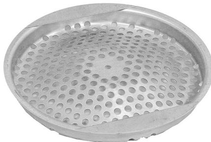
BH Filter bucket in stainless steel for Purus' Bigg and Heavy floor gullies. The filter bucket is used to collect particles larger than 5mm, such as leaves, so they do not fill up the water trap. The strainer can be removed for cleaning and maintenance.
