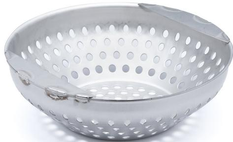
BH50 Filter bucket in acid-resistant stainless steel for Purus' Kitchen Channels and Bigg and Heavy floor gullies. The filter bucket is used to collect particles larger than 5mm, such as leaves, so they do not fill up the water trap. The strainer can be removed for cleaning and maintenance.
