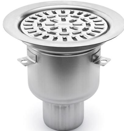
The Balder 75 R floor drain has a 75mm vertical outlet and is for installation in wooden or concrete joists. The Balder floor drain comes with a stainless steel water trap, clamping ring and stainless steel grate. It also comes with a protective cover that is intended to prevent any concrete or debris from installation from entering the drain.
