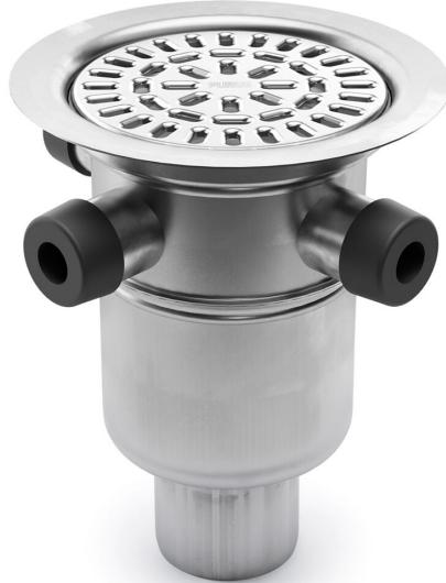
The Baldex 75 R floor drain has a 75mm vertical outlet and three extra inlets. Only one of the extra inlets should be used. The floor drain is suitable for installation in wooden or concrete joists and comes with a stainless steel water trap, clamping ring and stainless steel grate. It also comes with a protective cover that is intended to prevent any concrete or debris from installation from entering the drain.
