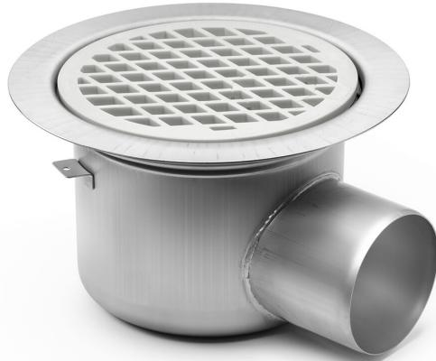
The Bigg 110 P floor drain has a 110mm side outlet and is for installation in concrete joists. The Bigg floor drain comes with a water trap, clamping ring and plastic grate. It also comes with a protective cover that is intended to prevent any concrete or debris from installation from entering the drain.
