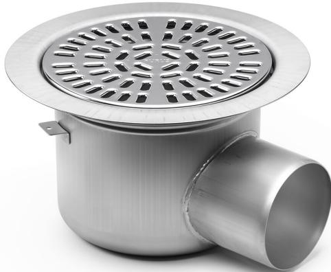
The Bigg 110 R floor drain has a 110mm side outlet and is for installation in concrete joists. The Bigg floor drain comes with a stainless steel water trap, clamping ring and stainless steel grate. It also comes with a protective cover that is intended to prevent any concrete or debris from installation from entering the drain.
