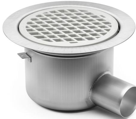
The Bigg 75 P floor drain has a 75mm side outlet and is for installation in concrete joists. The Bigg floor drain comes with a water trap, clamping ring and plastic grate. It also comes with a protective cover that is intended to prevent any concrete or debris from installation from entering the drain.
