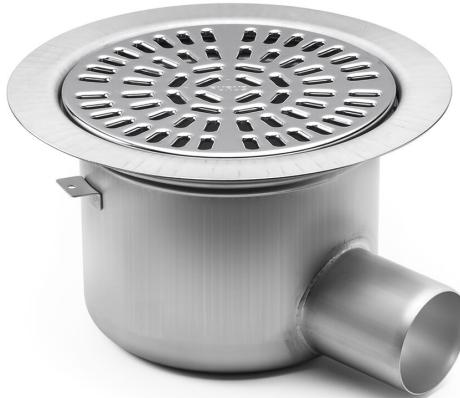
The Bigg 75 R floor drain has a 75mm side outlet and is for installation in concrete joists. The Bigg floor drain comes with a stainless steel water trap, clamping ring and stainless steel grate. It also comes with a protective cover that is intended to prevent any concrete or debris from installation from entering the drain.
