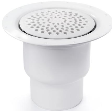
The Brage 110 Vertical floor drain has a 110mm vertical outlet and is for installation in wooden or concrete joists. The Brage floor drain comes complete with a removable water trap, clamping ring and plastic grate. It also comes with a protective cover that is intended to prevent any concrete or debris from installation from entering the drain.
