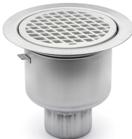
The Heavy 110 P floor drain has a 110mm vertical outlet and is for installation in concrete joists. The Heavy floor drain comes with a water trap, clamping ring and plastic grate. It also comes with a protective cover that is intended to prevent any concrete or debris from installation from entering the drain.
