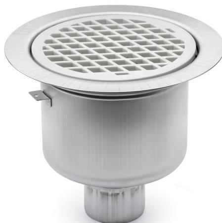
The Heavy 75 P floor drain has a 75mm vertical outlet and is for installation in concrete joists. The Heavy floor drain comes with a water trap, clamping ring and plastic grate. It also comes with a protective cover that is intended to prevent any concrete or debris from installation from entering the drain.
