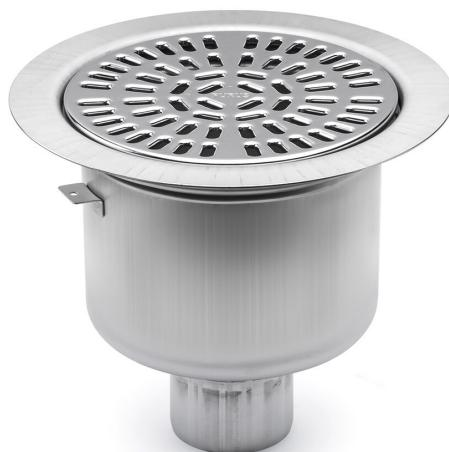
The Heavy 75 R floor drain has a 75mm vertical outlet and is for installation in concrete joists. The Heavy floor drain comes with a stainless steel water trap, clamping ring and stainless steel grate. It also comes with a protective cover that is intended to prevent any concrete or debris from installation from entering the drain.
