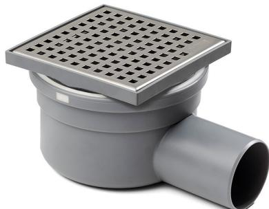
Floor Drain Kvaser has a 50mm side outlet and the floor drain can be cut to adjust the overall height between 85-120 mm. The floor drain comes complete with a NOOD water trap and stainless steel grate.
