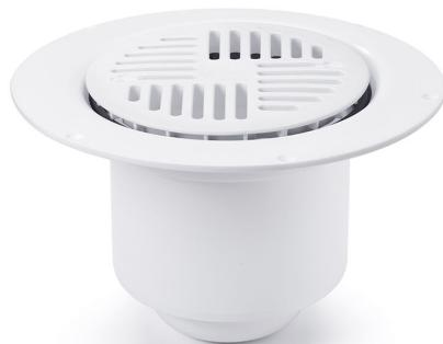
The Mini Brage 110 floor drain has a 110 mm vertical outlet and is suitable for installation in wooden or concrete joists. The Mini Brage 110 floor drain comes complete with a removable water trap, clamping ring and plastic grate.
