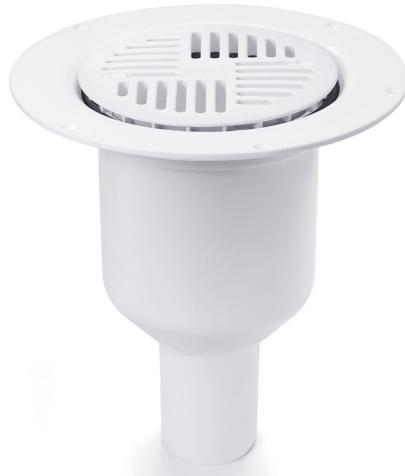
The Mini Brage 50 floor drain has a 50 mm vertical outlet and is suitable for installation in wooden or concrete joists. The Mini Brage 50 floor drain comes complete with a removable water trap, clamping ring and plastic grate.
