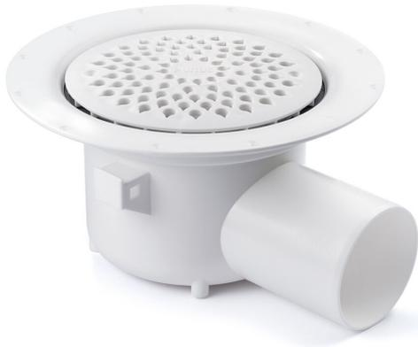
The Oden floor drain has a 75mm sideoutlet and is for installation in wooden or concrete joists. The Oden floor drain comes complete with a removable water trap, clamping ring and plastic grate. It also comes with a protective cover that is intended to prevent any concrete or debris from installation from entering the drain.
