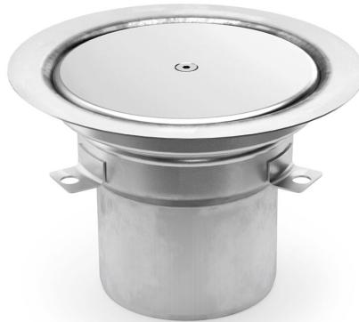
The Rens 110 R untrapped floor drain has a 110 mm vertical outlet and is for installation in concrete joists. The Rens comes with a stainless steel lockable cover which is load-bearing up to 1.5 tons. It also has a tight plastic inner lid.
