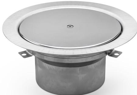
The Rens 160 untrapped floor drain has a 160mm vertical outlet and is for installation in concrete joists. The Rens comes with a stainless steel lockable cover which is load-bearing up to 1.5 tons. It also has a tight plastic inner lid and a ring to accommodate water traps.
