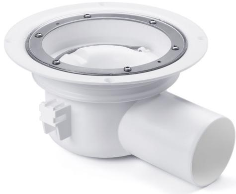
The S-Series Oden is a floor drain with a 75mm side outlet for installation in wooden or concrete joists. The S-Series Oden floor drain comes with a removable water trap and stainless steel clamping ring. It also comes with a protective cover that is intended to prevent any concrete or debris from installation from entering the drain.
