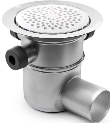
The Sigex 75 P floor drain has a 75mm side outlet and three extra inlets. Only one of the extra inlets should be used. The floor drain is suitable for installation in wooden or concrete joists and comes with a water trap, clamping ring and plastic grate. It also comes with a protective cover that is intended to prevent any concrete or debris from installation from entering the drain.
