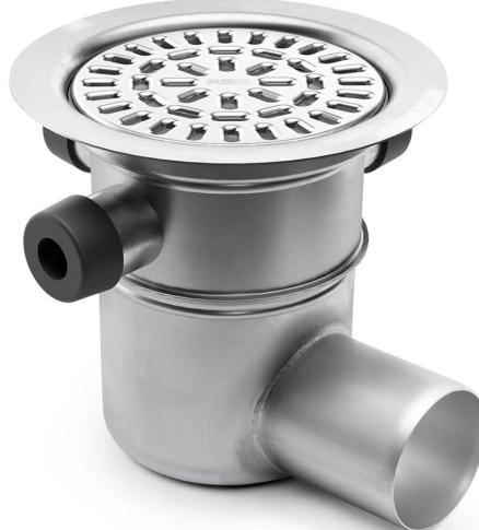
The Sigex 75 R floor drain has a 75mm side outlet and three extra inlets. Only one of the extra inlets should be used. The floor drain is suitable for installation in wooden or concrete joists and comes with a stainless steel water trap, clamping ring and stainless steel grate. It also comes with a protective cover that is intended to prevent any concrete or debris from installation from entering the drain.
