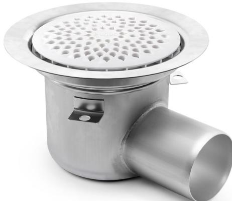
The Sigyn 75 P floor drain has a 75mm side outlet and is for installation in wooden or concrete joists. The Sigyn floor drain comes with a water trap, clamping ring and plastic grate. It also comes with a protective cover that is intended to prevent any concrete or debris from installation from entering the drain.
