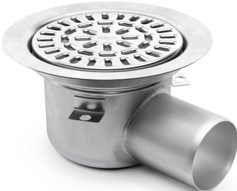
The Sigyn 75 floor drain has a 75mm side outlet and is suitable for installation in wooden or concrete joists. The Sigyn floor drain comes with a stainless steel water trap, clamping ring and stainless steel grate. It also comes with a protective cover that is intended to prevent any concrete or debris from installation from entering the drain.
