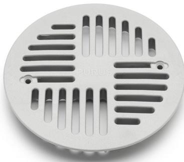
The Art Deco 130 is made of 100% recycled plastic in grey. For Purus floor drains with a 130mm grate diameter. It is suitable for vinyl floor finishes. The grate is designed to withstand a good flow rate and has a K3 load class.
