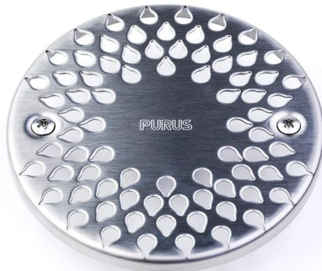
Floor gully Drop 130 is a grate made of durable stainless steel. Fits all Purus floor gullies with grate dimension 130mm. The grate is manufactured to ensure a good flow rate and has load class K3. Included with a locking device with a stainless steel locking bracket designed to lock the grate down by attaching to the clamping ring underneath.
