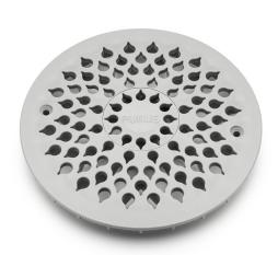
The Drop 150 is made of 100% recycled plastic in grey with cutouts for up to 40 mm outlet pipe. Fits all Purus floor drains with stainless steel clamping ring. The grate is designed to withstand a good flow rate and has a K3 load class.
