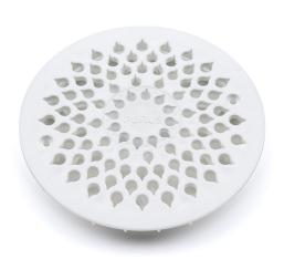
The Drop 150 is a plastic grate with a 40mm diameter inlet for pipes. It fits all Purus floor drains with a 150mm grate diameter, and is suitable for vinyl floor finishes. The grate is designed to withstand a good flow rate and has a K3 load class.
