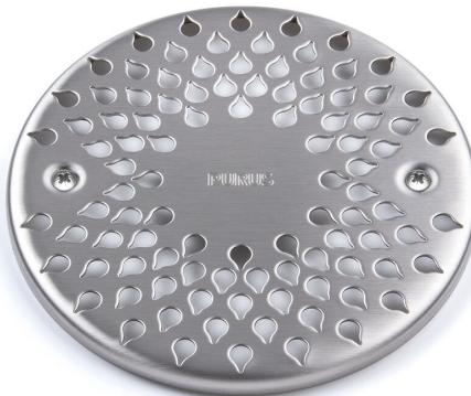
Floor gully Drop 150 is a grate made of durable stainless steel. Fits all Purus floor gullies with grate dimension 150mm. The grate is manufactured to ensure a good flow rate and has load class K3. Included with a locking device with a stainless steel locking bracket designed to lock the grate down by attaching to the clamping ring underneath.
