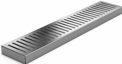
Rib is made of stainless steel. Rib is a non-slip grid with load class K3 (300 kg) for walking traffic/barefoot friendly. Dimensions 100×500 mm.
