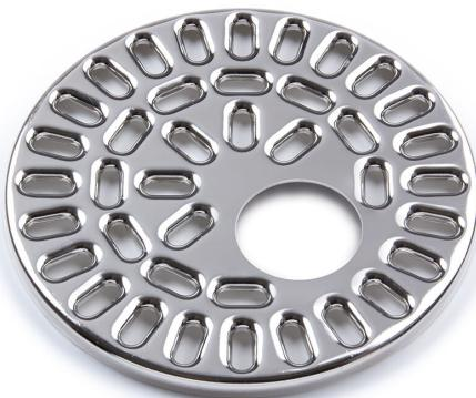
The SR 150 grate is made of acid-resistant stainless steel, has a 40mm diameter inlet and is designed for use with Purus' 150mm diameter floor drains. It is suitable for vinyl floor finishes and has a K3 load class.
